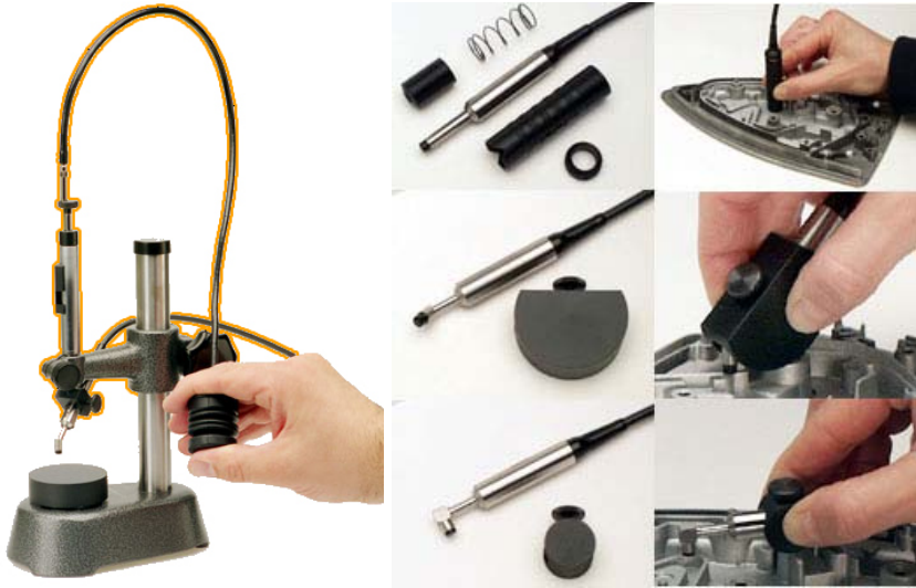
Fig. 6: Positioning device (left) and various positioning aids (right) for the micro probe
